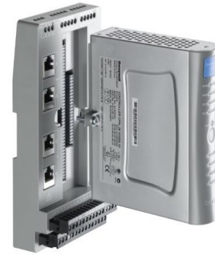
Figure 5. RTU Processor ease of removal from IOTA
